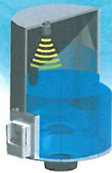
■Liquid level measurement
