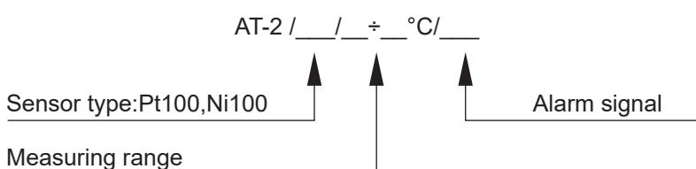
Example: temperature transmitter AT-2, sensor type Pt100, measuring range 0...100°C, alarm signal 22mA.
