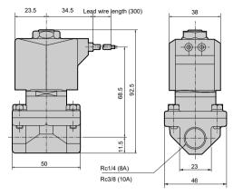
\*1: The dimensions are the same for the G or NPT thread port size.
